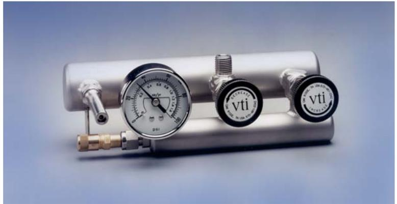
The RLS has a reservoir of liquid refrigerant that is interconnected with a valve to the vapor reservoir to provide a convenient, long time supply of vapor for the Leak. Depending on use patterns and QA requirements, these Leaks are typically sent to VTI for refill and recalibration after one to three years of use. Unlike the fragile glass capillaries sometimes used by other manufacturers, the RLS uses a crimped stainless-steel capillary leak element that is unbreakable.
